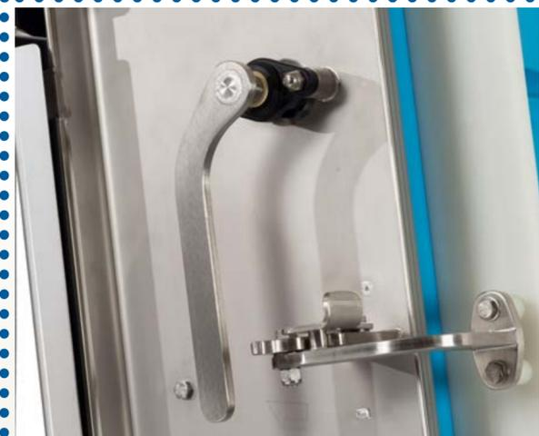
Manual belt lifters enable easy access for cleaning
