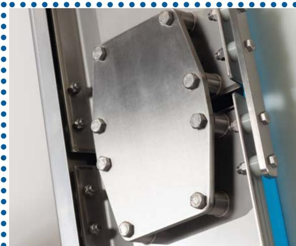
All wash-down duty components mounted on stand offs to meet sanitation requirements
