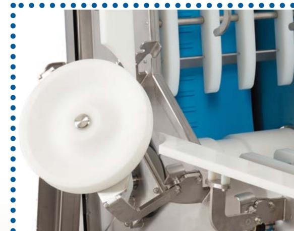
Fold out, rounded UHMW wheels to assist belt tracking.
