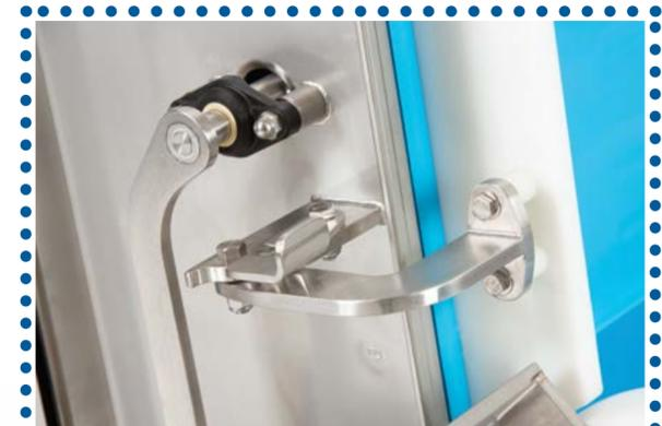
Quick release UHMW side boards mounted on hinges, captivated to conveyor frame. Eliminate potential for lost/misplaced guides during sanitation process.
