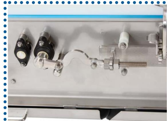
Easy to operate, belt tensioner to loosen belt prior to removing sideboards and activating belt lifting system
